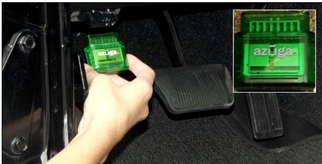
Figure 36: MRD installation to the OBD-II Port
